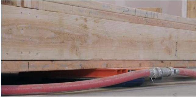
*Factory magic: the AeroGo air caster system uses compressed air to lift, float and move structures up to 70,000 lbs.*
