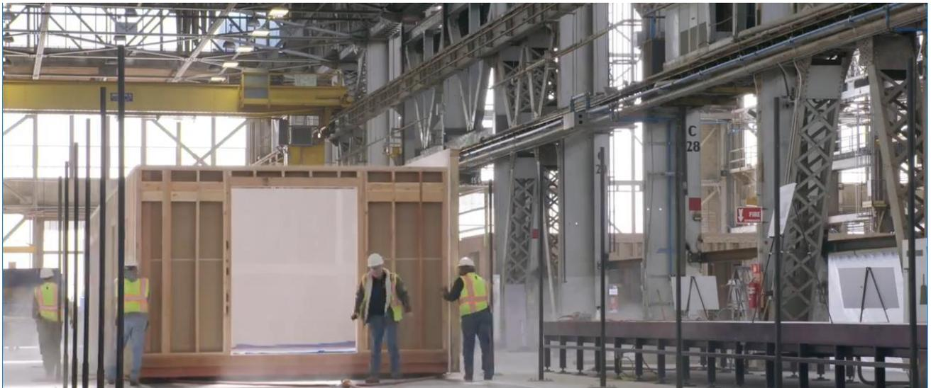
*Pre-fab structures float on air bearings as they progress through 30 assembly workstations.*
